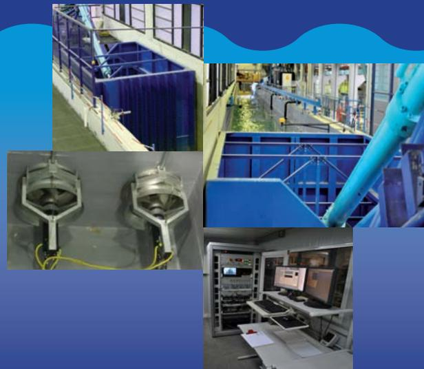
The control software allows regular and irregular waves (e.g. parametric or user-defined spectra and measured time series) to be generated. Additionally, a PC-based active absorption system allows tests to be run on wave series for as long as required, without the effect of spurious model-induced reflections. This is an essential feature for testing highly reflective structures and for analyzing equilibrium shapes in beach profiles, particularly accretive sequences.
